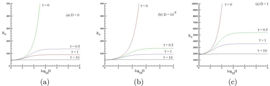
Figure 1: Critical Rayleigh number as a function of  $H$  for various values of  $\gamma$ . a)  $D = 0$ , b)  $D = 10^{-3}$ , c)  $D = 10^{-3}$ .
