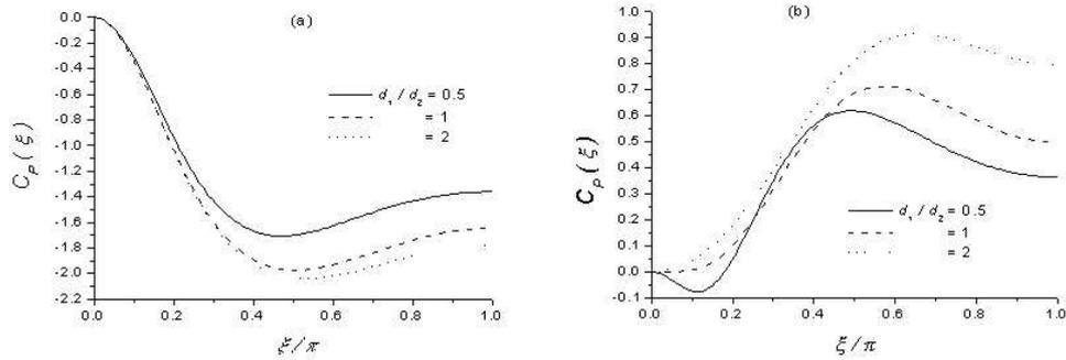
Figure 5: The distribution of the pressure coefficient over the bodies surface;  $2 L_1 / d_1 = 2$ ; (a) upstream cylinder; (b) downstream cylinder.
