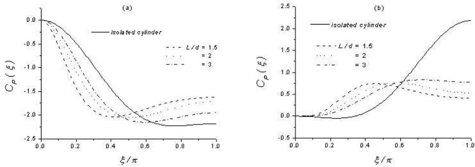
Figure 3: The distribution of the pressure coefficient over the bodies surface;  $d_1 = d_2 = d$ ; (a) upstream cylinder; (b) downstream cylinder.
