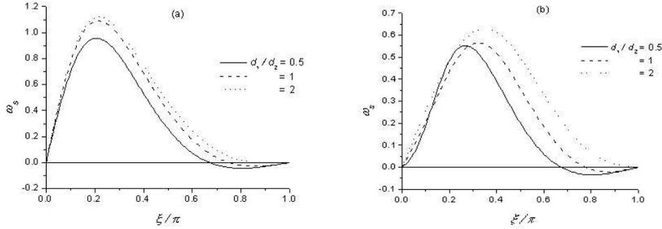
Figure 4: The distribution of the vorticity over the bodies surface;  $2 L_1 / d_1 = 2$ ; (a) upstream cylinder; (b) downstream cylinder.
