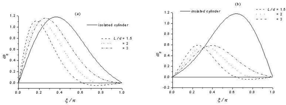
Figure 2: The vorticity distribution over the bodies surface;  $d_1 = d_2 = d$ ; (a) upstream cylinder; (b) downstream cylinder.
